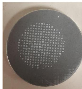
Fig. 2. Photograph of micropatterned aluminium substrate
